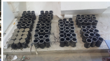
c) Cylinder type specimen for concrete strength
